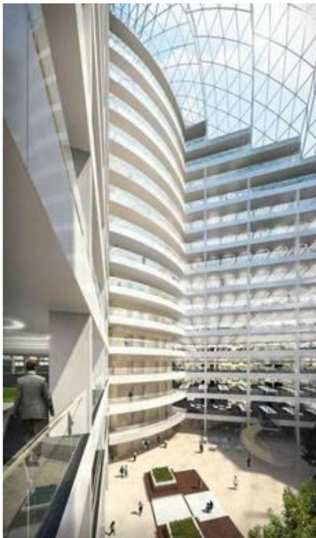
The building's double skin facade helps minimise heating and cooling loads. In summer louvres at the top of the facade open to allow the warmed air trapped between its inner and outer skins to rise up and out of the building. In winter these louvres are closed so the facade can form an insulated blanket around the building.
