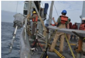
*Coring machine used to gather sediment samples from the Pacific.
